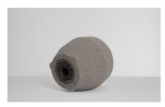
Specifically designed for use in hand moulding. The elimination of the traditional breaker ensures optimised, and reliable feeding of the casting due to the increased contact of the riser at the casting. Easy riser removal is ensured due to the addition of the refractory mesh and the predetermined fracture point within the riser neck.
