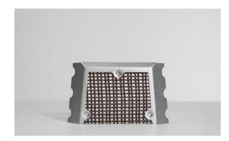
The NETFrame\* has been specially designed for the removal of large side risers. It is positioned into the riser neck adjacent to the casting surface where the refractory mesh ensures a defined and predetermined fracture point ensuring easy removal of the riser.
