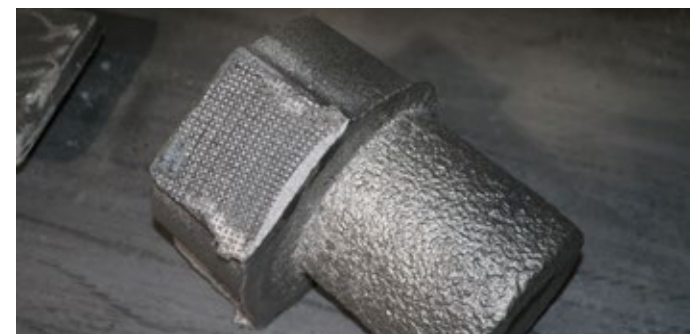
Riser rest after knocking off
