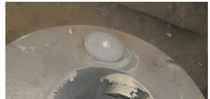
NETCore® casting before cleaning process (riser residue knocked off)
